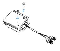
9. Secure the front of the metal cover with the long screw that you removed in step 2
